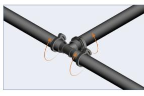
Pinch ratchet clamps & check for leaks
