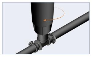
Hand tighten & check for leaks
