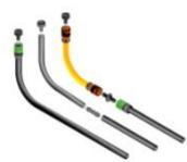
A soaker hose can be connected to the tap in three ways. Direct connection is the most simple, however does allow water wastage from the soaker hose before it reaches where it is required to water. Use either **LDPE** or **Garden Hose** to take water directly between flower beds or planters.
