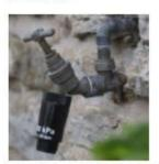
Soaker hoses are perfect for domestic garden environments as they operate under low pressures (between **0.5 - 1 bar**). To maintain an even level of watering along the length of the hose, you will need a **Pressure Reducer** to ensure water from your hose is seeping, not spurting. Pressure reducers can be easily installed directly to a <sup>3</sup>/<sub>4</sub>" garden tap followed by your tap connector and chosen method of supply.
